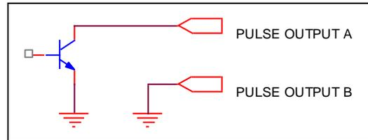
Some consoles and card systems are not compatible with the open collector pulse output, while nearly all are compatible with contact closure pulsers. Consult the wiring diagrams for your particular console or card system model. The PA2 pulse analyzer will operate with either type.
