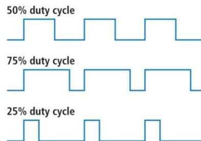
The duty cycle value is only valid when the pulses are being sent continuously. Duty cycles with values below 25%, or greater than 75% may indicate a problem for some consoles or card systems where the frequency of the pulses approaches the maximum input speed. The duty cycle is displayed on the PA2 as DC>00, where the value can range from 00 to 99.
